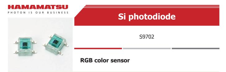
The S9702 is a color sensor molded into a plastic package having a 3-channel (RGB) photodiode sensitive to the blue ( $\lambda p$ =460 nm), green ( $\lambda p$ =540 nm) and red ( $\lambda p$ =620 nm) regions of the spectrum. The S9702 has a 3-segment (RGB) photosensitive area of  $\Box 1$  mm. When compared to the previous model (S9032-02), the S9702 is significantly miniaturized (package size 55% less in cubic volume, PC board mount space 43% less in area).
